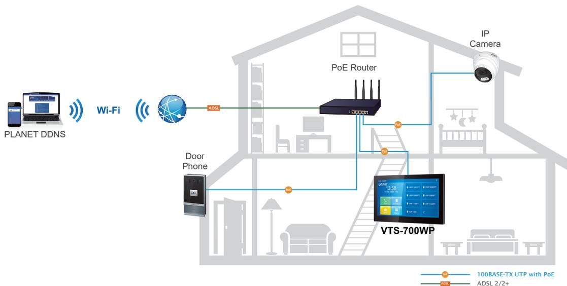
The system utilizes a 7" Touch Screen to get to the key functions with just one click to combine various household facility applications, including camera monitoring, access control, intercom, security, scene control, and value-added services, to bring you a new, comfortable and convenient lifestyle.
