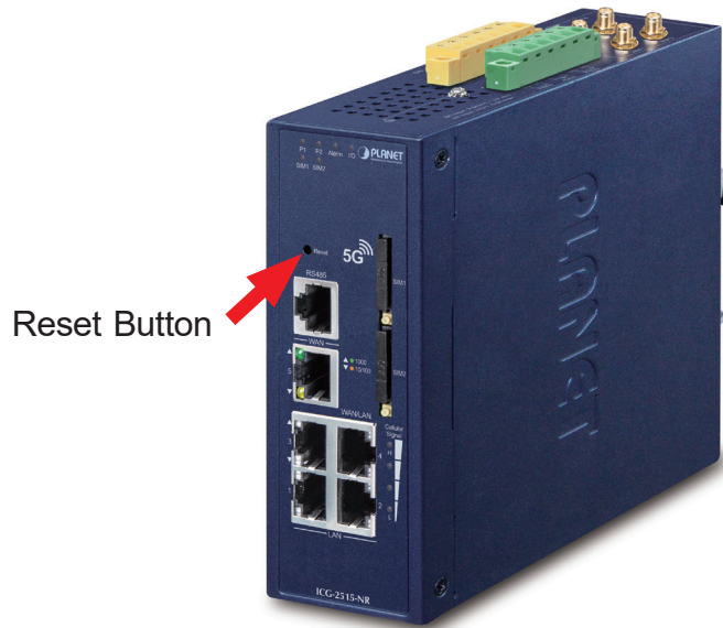
Figure 5-1: ICG-2515 Series Reset Button
