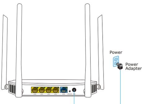
**Step 3:** Follow the figure below to connect the network devices. It depends on your network environment to connect the WAN port to a Cable/xDSL modem, or the Ethernet directly in your place.
