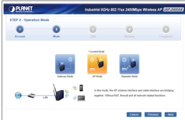
Figure 4-3: Web Wizard Operation Mode of Industrial 802.11ax Wireless AP
