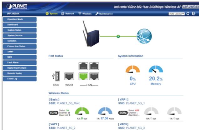
Figure 4-4: Web Main Screen of Industrial 802.11ax Wireless AP
